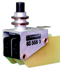
Telescopic plunger with Ø10 mm threaded barrel, metal bracket and plastic button. Single or double pole (83556)
