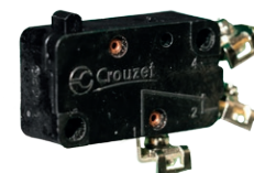
Customised version for nuclear application. Has radiation-resistant housing, 180 °C max operating temperature, W5 screw terminals and magnetic blowout for highly inductive circuit switching at 250 V...
