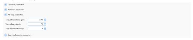
Set the PID controller factors in the torque control loop (this function is reserved for advanced users). The values given in the example below ensure correct product operation in the majority of cases.
