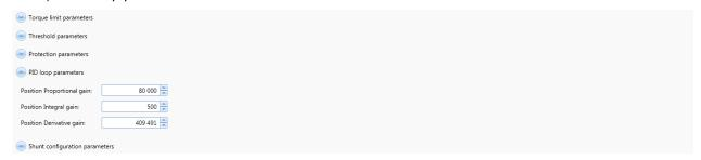
Set the PID controller factors in the position control loop (this function is reserved for advanced users). The values given in the example below ensure correct product operation in the majority of cases.
