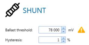
The external shunt will be activated when the actual bus voltage is higher than **Ballast threshold** plus **hysteresis** and will be deactivated when the actual bus voltage is lower than **Ballast threshold** minus **hysteresis**. This **hysteresis** is expressed as percentage of Ballast threshold.
