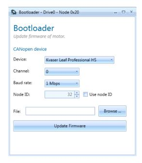
Select the .hex file that you want to load inside the SMI21 or SMI22 CANopen drive by click on the "Browse" button and after click on the "Update Firmware" button to launch the bootloader sequence.
