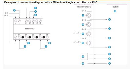
NB: The "tachometer" and "actual direction of rotation" card outputs must be connected to inputs i1 and i2 respectively in order to be able to use the Motomate high-speed counter function.
