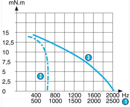
Inertia of measuring chain : 1,5 g.cm2 a = constant voltage controller with Rs (resistance in series) = 0 b = constant voltage controller with Rs (resistance in series) = R motor c = constant voltage controller with Rs (resistance in series) = 3R motor The measurements are made with full stepping, 2-phases energised.
