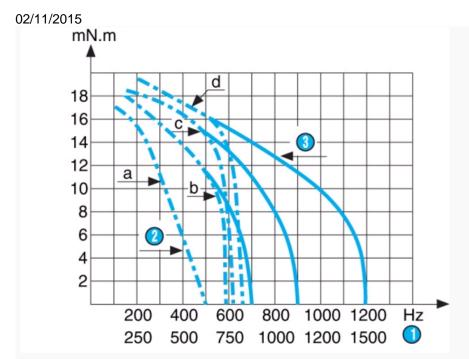
Inertia of measuring chain : 1,5 g.cm2 a = constant voltage controller with Rs (resistance in series) = 0 b = constant voltage controller with Rs (resistance in series) = R motor c = constant voltage controller with Rs (resistance in series) = 3R motor The measurements are made with full stepping, 2-phases energised.
