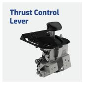
Intuitive design that allow pilots to maintain manual controls for the complete control over their aircraft's thrust systems with ease
