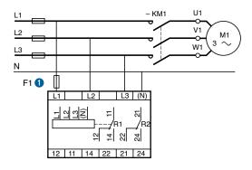
100 mA fast-blow fuse or cut-out
