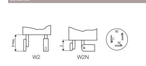
Electrical diagram (actuator at rest position)
