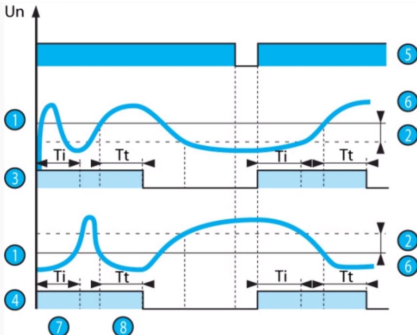
If "with memory" mode has been selected, the relay opens and stays in this position when threshold crossing is detected. The power supply must be disconnected to reset the product.
