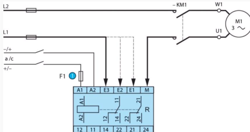
NB : When controlling DC current from the same source supplying terminals A1 and A2, terminal M must be connected directly to the "minus" pole of this power supply.
