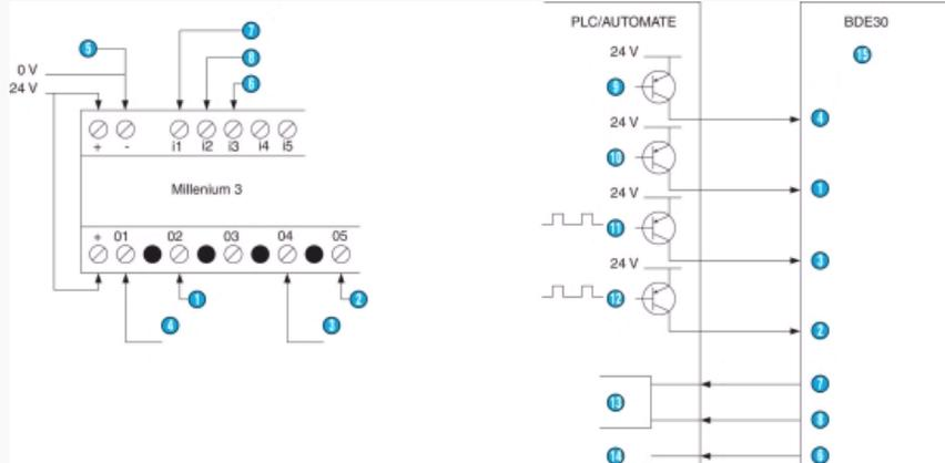
NB : The "tachometer" and "actual direction of rotation" card outputs must be connected to inputs i1 and i2 respectively in order to be able to use the Motomate high-speed counter function.
