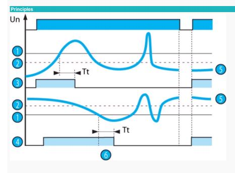
The under or overvoltage threshold value is set by a graduated potentiometer by reading the Un scale to be monitored directly.
